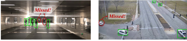
(a) Detect with Low Resolution (b) Detect with Low Frame Rate Fig. 2. Inappropriate Configurations for Detecting Objects
